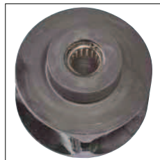
Load chain sheave with needle bearing
